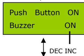
The beep sounds at every time pressing the buttons to confirm your action. The beep or melody sounded at various times during operation to alert different mode changes. These audible sounds can be on or off.
