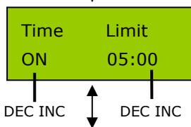
When you start a charge process, the integral safety timer automatically starts running at the same time. This is programmed to prevent overcharge the battery if it proves to be faulty or if the termination circuit can not detect the battery full charged. The value should be generous enough to allow a full charge of the battery. The time format is hh:mm.
