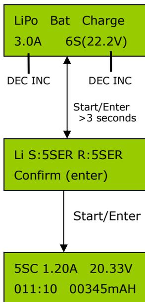
The value on the second line sets a charge current and the voltage of the battery pack. Press the **STATR/ENTER** button, and then press the **DEC or INC** to set value. After setting the current and voltage press **STATR/ENTER** button for more than 3 seconds to start the process. (Charge current: **0.1~8.0A**, Voltage: 1~6 series)
