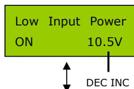
The program monitors the voltage of battery used as input power. If the voltage drops below the value you set, the charging process will be terminated forcibly to protect the battery.
