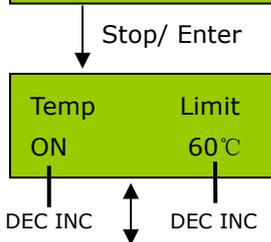
An optional feature using temperature probe contacts the surface of battery. The feature can be on or off. If it is on, set the maximal temperature at which the charger allows battery to reach during charge. Once the battery temperature reaches the limit while charge, the charging will be ended to protect the battery
