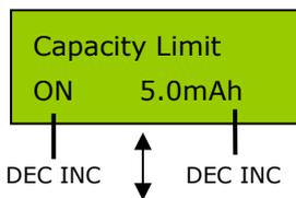
The program sets the maximal charge capacity that will be supplied to the battery during charge. If the termination circuit can not detect the battery full charged, this feature will automatically stop charging at the set capacity value.
